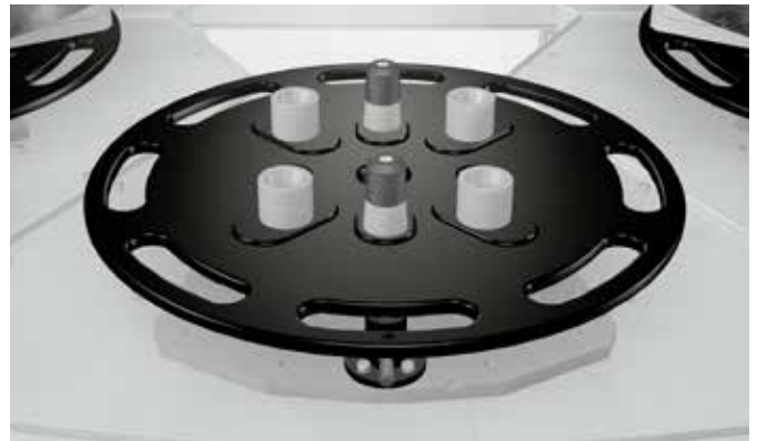
Rotatable magazine plates simplify setup and preparation. Pre-centering facilitates pallet positioning with crane and LiftGear.
