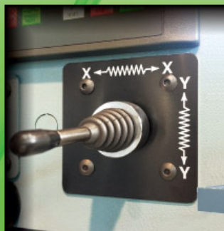
X、Y軸手動操控自動進給 X,Y axis manual control then automatic feed
