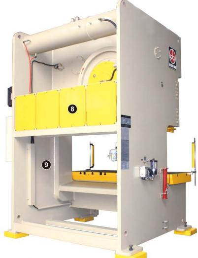
8. 油壓超負荷裝置 Hydraulic overload device
