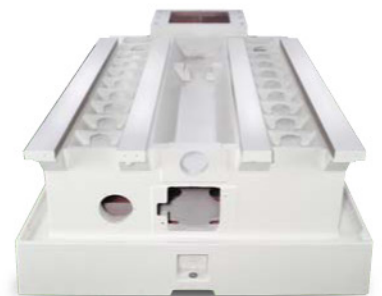
One Piece 4-Boxway in Y-axis ( CINCH-Mill 50/60 )
