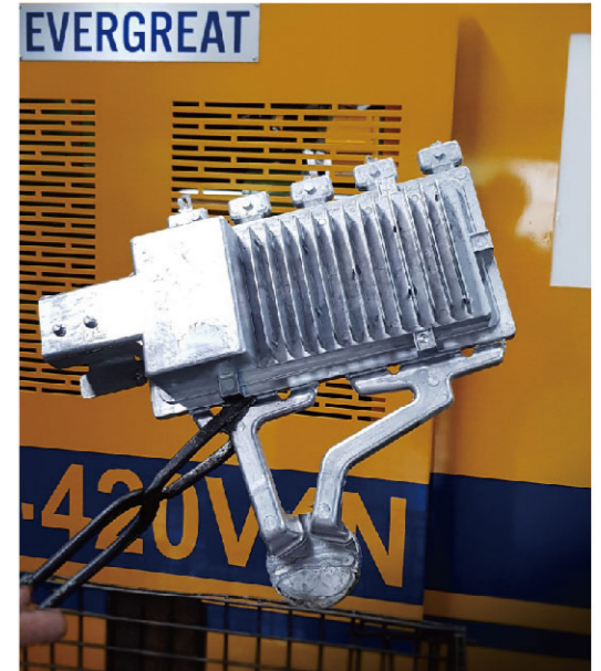
Die-casting trial samle DC420V4N測試
