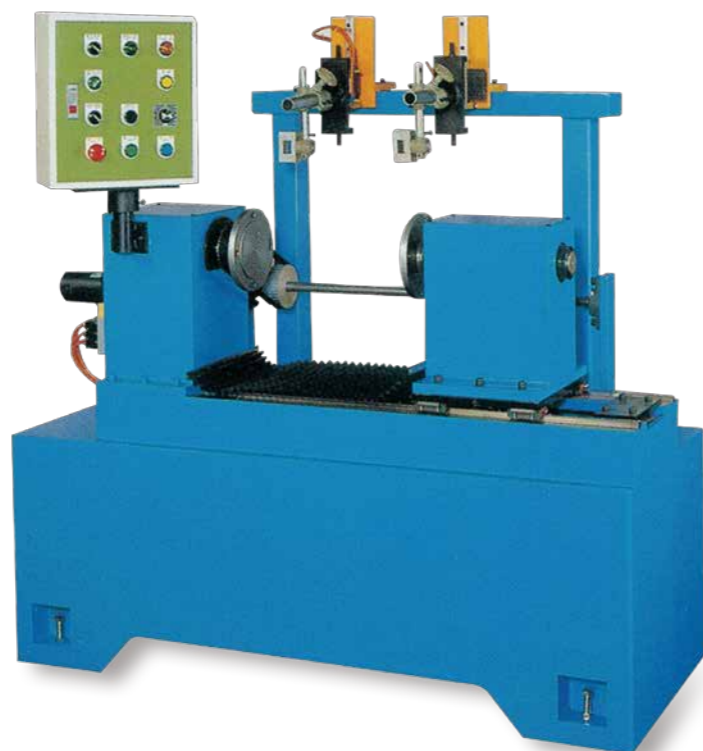
DJ-N III 300~1200 Double Gun Type Straightening Burning Weld Auto Table 雙槍直線燒焊自動台
