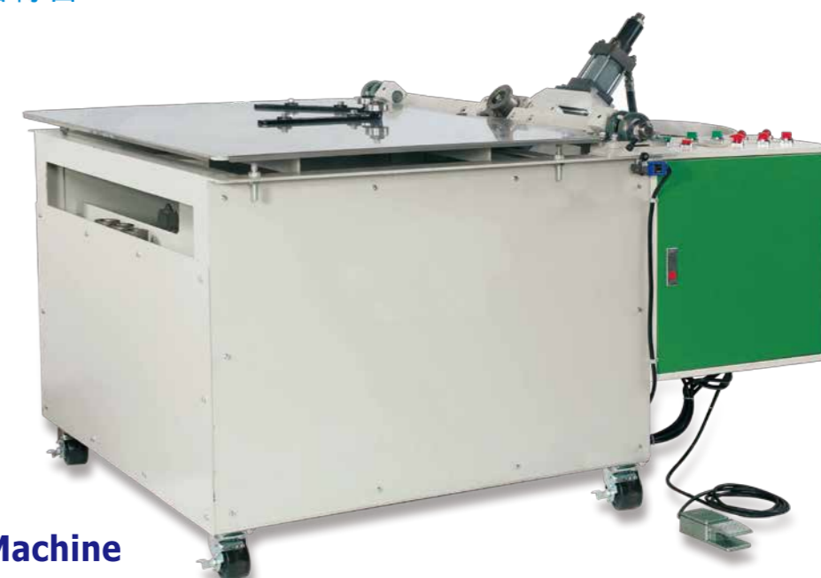
DJ-O I 50~500 Horizontal Type Single Gun Auto Burning Weld & Auto Rotating Table 單槍臥式自動燒焊回轉台
