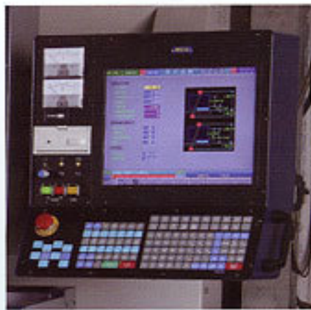
120° 可移動式操作面板，符合人體工學 120° swivel movable panel fit for ergonomics.
