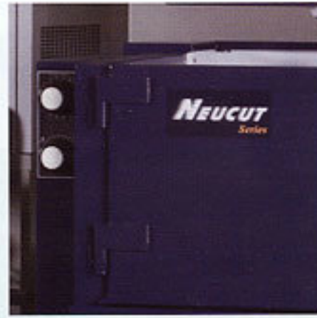
旋鈕式液位&閘門開關，操作方便 Knob switch to control level and inlet gate of fluid.
