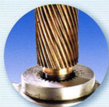
Slanting gear wheel machining
