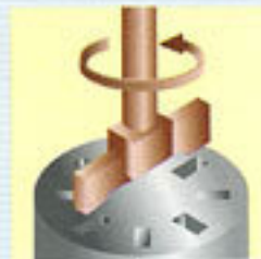
C-axis rotation angle positioning machining
