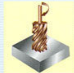
C-axis thread machining
