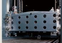
The beam is clamped securely by hydraulic force in combination with the use of disc springs. This fully prevents the beam from slipping down to eliminate any loss in grinding accuracy.
