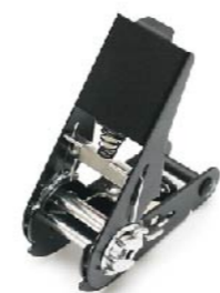
1" Aluminum Ratchet Bukcle RBA24-001 Size: 1"/25mm B.S: 500kg Finish: Anodized
