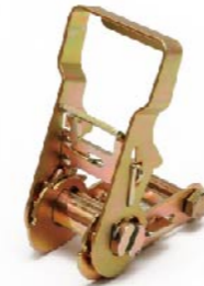
1" Once Forming Frame Ratchet Buckle RB28-010 Size: 1"/25mm B.S: 1200kg Finish: Yellow Zinc Handle and side panel once forming type
