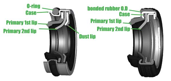
**Primary 1st lip** : to prevent refrigerants leakage when shaft rotating. HNBR has effective resistance against refrigerants and refrigeration lubricants and also has excellent temperature resistance range from -40°C to 150°C.
