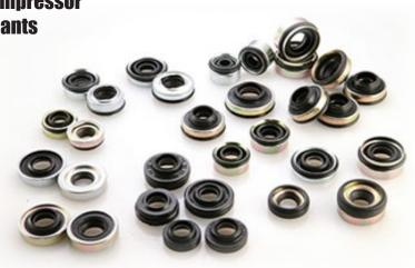
WSI automotive air conditioning compressor seals are composed of a metal case with adhesion of a primary 1st lip made of HNBR and a primary 2nd lip made of PTFE. Most of these seals are incorporated with an O-ring or bonded rubber O.D. for static sealing and proper installation.
