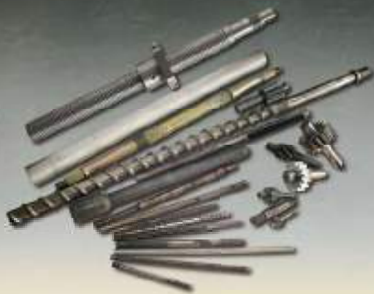
滾珠螺桿、棒管類整直樣品 Straightened Sample of Ballscrew, Rods and Pipes
