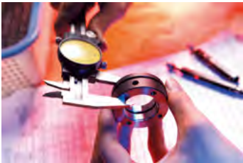
We measure the thickness of the locknut. (refer to photo)
