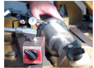
We measure the locknut thread run-out. (refer to photo)
