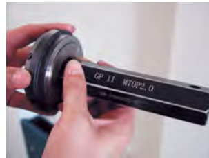
We check the thread precision by a gauge to insure ISO 4H. (refer to photo)
