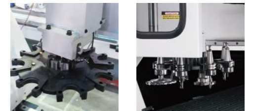
傘型刀庫(工作到哪可馬上換刀，讓效率更高) Drum type ATC ( When the machine work in any position can change the tool immediately, higher efficiency)
