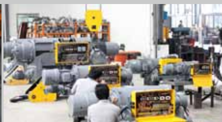
鋼索吊車組裝廠區 & 電控測試區 Assembly Line of Electric Wire Rope Hoists & Control Panel Testing Line
