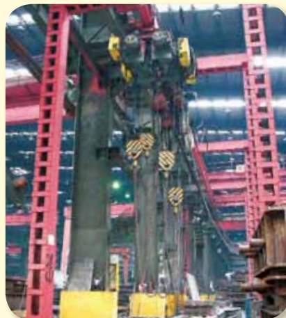
鏈條吊車 適用：塑膠組裝加工廠 Electric Chain Hoist in Plastic Assembly Plant
