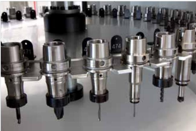
**Tool Checking** | Besides the workpieces and NC programs, you need the right tools as well. Whether this is the case, and what their remaining lives are, is read from the memory of the machine.
