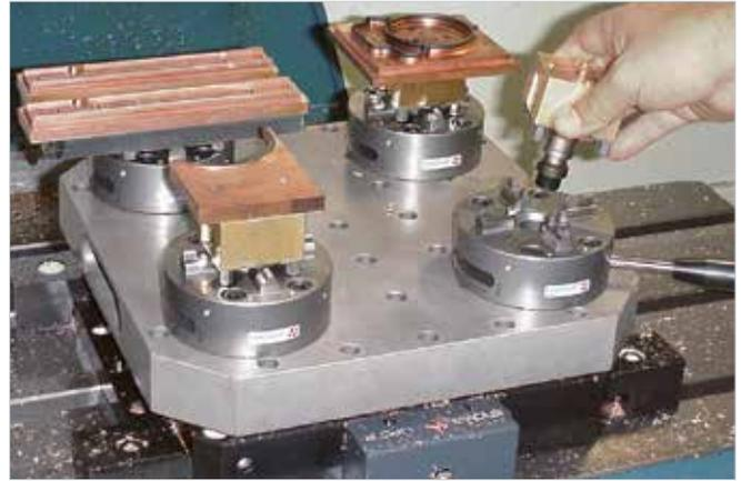
**Fixture Manager 1** Manages several fixtures on a pallet, automatically storing the position of a clamped workpiece. The identification system ensures the correct matching of the data.
