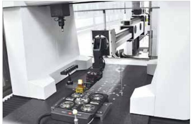
**More capacity |** Even the "quality measurement" process step can be automated. A potential bottleneck is eliminated by automatic measurements in the second and third shifts.
