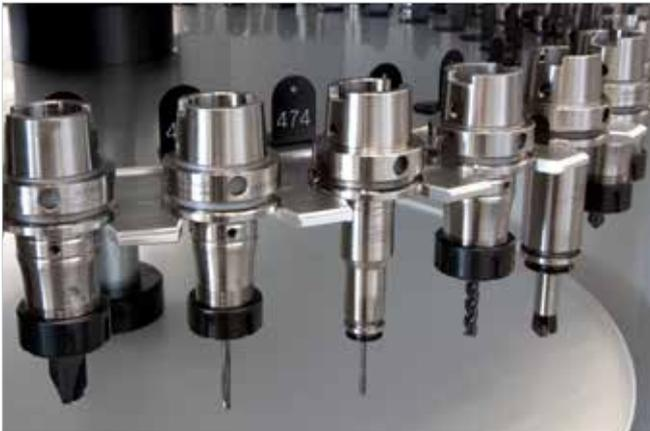
**Tool Checking 1** The ToolManagement module checks which tools are required based on the NC program right after a job has been created. A comparison with the tool list of the machine shows whether the job can be released or not.
