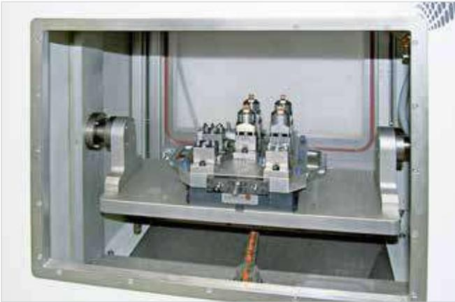
**Cleaning |** The "washing/cleaning" production step is necessary if several processes run in succession automatically. For example, workpiece milling > washing > measuring > EDM.
