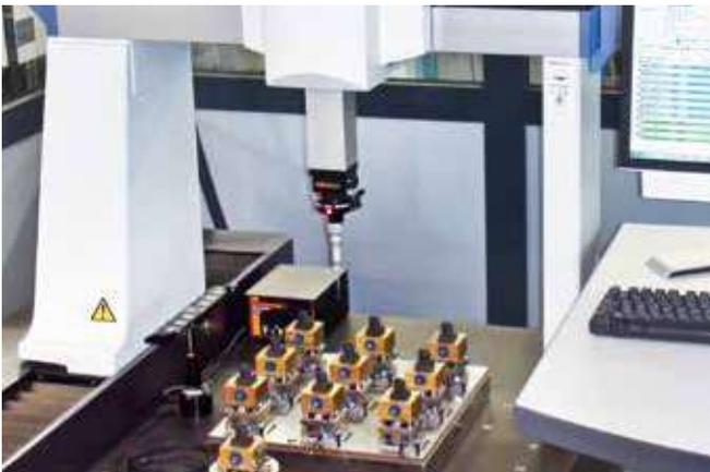
**Automatic presetting |** The larger the number of produced electrodes, the more important efficient measurement of zero points becomes.
