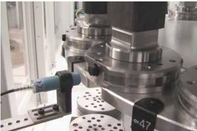
**Identification** | Staged pallets with workpieces are uniquely marked with a chip. At every station in the production process, each pallet is precisely identified by the EROWA EWIS™ system.
