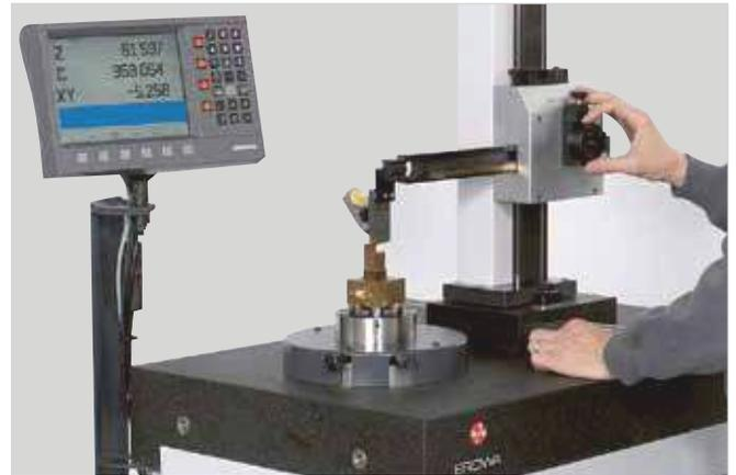
**Presetting** | Offset data of electrodes is determined easily on the PreSet 2D presetting station. The data is associated with the corresponding electrode through the integrated interface.
