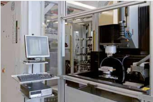
**The cell** | A production cell consists of the machine, the EROWA robot and the terminal for the process control system. By this, the operator has everything under control.
