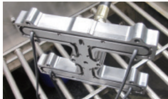
分流板流道拋光 Polishing of Manifold Runners
