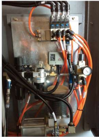
Lubrication and Pressure System
