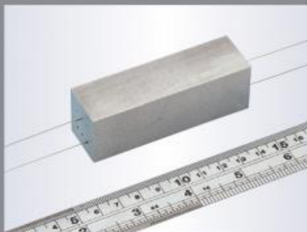
Material: Aluminum Thickness: 80mm Diameter: \varnothing 0.5mm
