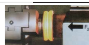
Heating and forging with a higher axial force applied.
