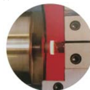
High-speed rotation from two sides to pressure and to make two workpieces tightly jointed.
