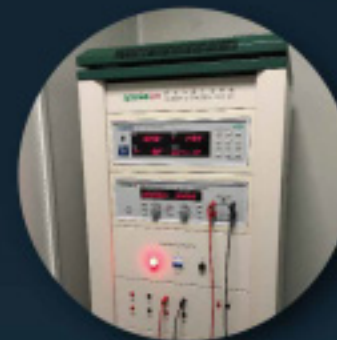
Control system (Measurement Station, Power Supply, Photometer)
