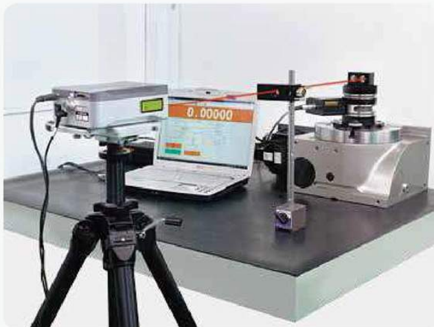
Renishaw laser instrument is applied for inspecting indexing accuracy.
