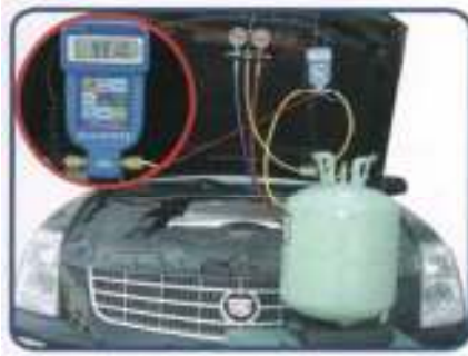
Charging for auto A/C system
